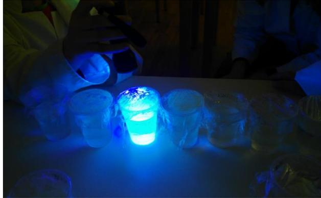
Label the plastic glasses as in the table below. Fill tonic water into four cups (approx. half full) and water into the last cup. Place cling film on top of each cup and cover three of them with the different substances (sun-cream, olive oil, cotton napkin). One cup with tonic water and the cup with normal water are only covered with the cling film. Irradiate each cup with the different types of lamps and observe.
