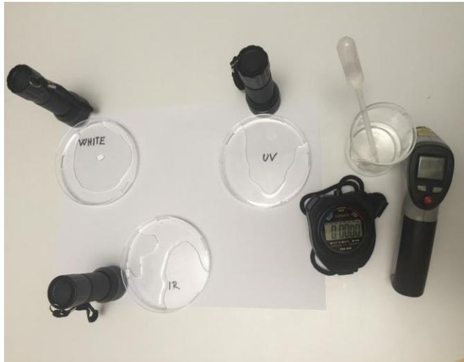
Write “white”, “infrared” and “ultraviolet” on the petri dishes. Add a small and equal amount of water into each petri dish. Use a thermometer to measure the starting temperature. Write down the number. Then, start irradiating each petri dish with the specific light for 4 minutes, then measure the water temperature again and write the numbers down. Wait another four minutes and measure again. Use a stopwatch to measure the time.
